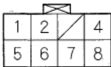
Wire side of female terminals
